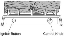
Figure 20 - Control Knob and Ignitor Button Location
